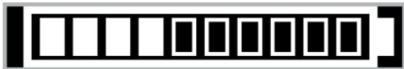
3. The solid segments of the battery show the current charge of the battery. The cycling segments of the battery highlights the proportion of the battery total capacity that has yet to be charged.
