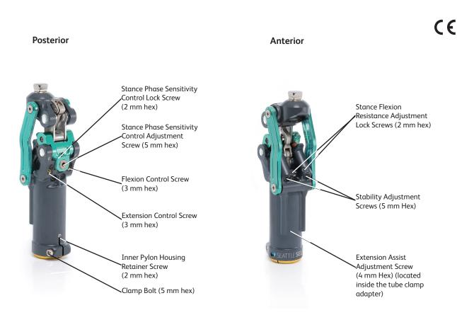
Figure 1. SSK615 and SSK615-THR Knee adjustment locations (SSK615 Select Stance Flexion Knee shown).
